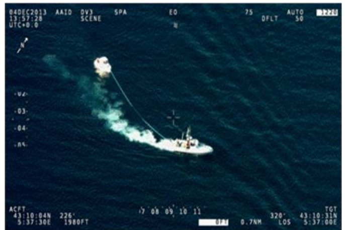
Fig. 26. INSPECTOR by ECA towing automatically a crippled boat
