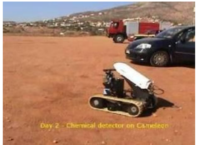
Fig. 25. CAMELEON by ECA with Chemical sensor on top
